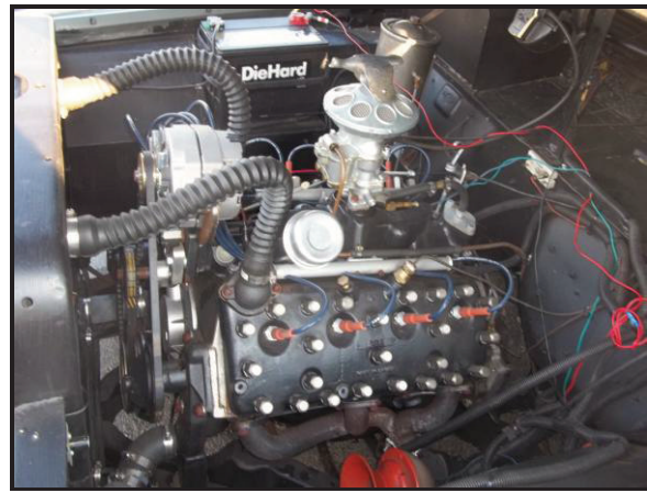
49 FORD FLATHEAD POWER (since this picture was taken A Rochester 4 barrel carb has been added)
